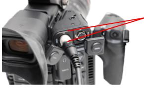
Align the **A** marks on cables' plugs and terminals
