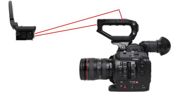
• Using the two supplied unit cables, connect the camera's AUDIO terminal to the monitor unit's AUDIO terminal and the camera's VIDEO terminal to the monitor unit's VIDEO terminal.
